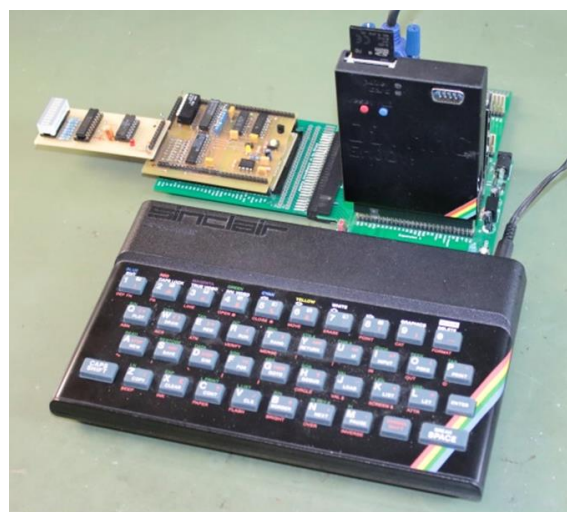
The total work of art: PIO, ZX-VGA, DivMMC - all mounted on the ProjectSPECCY backplane.
